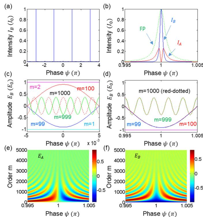
**Figure 2.** Numerical calculations for Equation (2). (a,b) Output intensities. (c–f) Output amplitudes. Amplitudes and intensities are normalized. Reflection coefficient is set at  $r = 0.999$ . The ring laser gain is not included. FP: Fabry–Perot interferometer.
